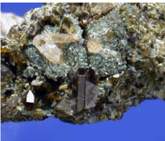
Epidote and quartz crystals in a cavity after calcite is removed with acetic acid. Epidote crystal in front right is 6 mm tall and only a portion of this crystal was exposed before cleaning. Salida Copper Mine, Chaffee County, Colorado. Julian C. Gray, photograph and specimen.
